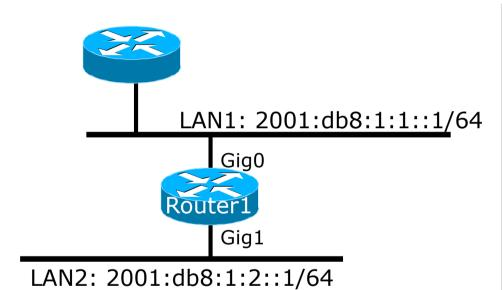
Dual stack IPv4/IPv6 single topology configuration.
