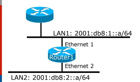
Dual stack IPv4/IPv6 single topology configuration.
