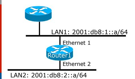
Dual stack IPv4/IPv6 multitopology configuration.
