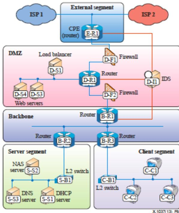
Figure 6-1 – Example topology of an IPv6 enterprise network
