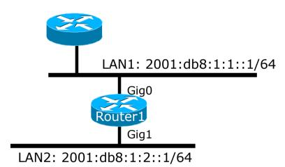
Dual stack IPv4/IPv6 single topology configuration.
