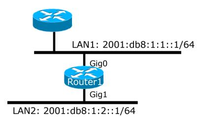
Dual stack IPv4/IPv6 multitopology configuration.
