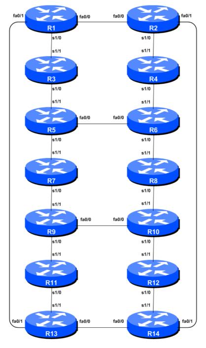
Figure 1 – ISP Lab Basic Configuration
