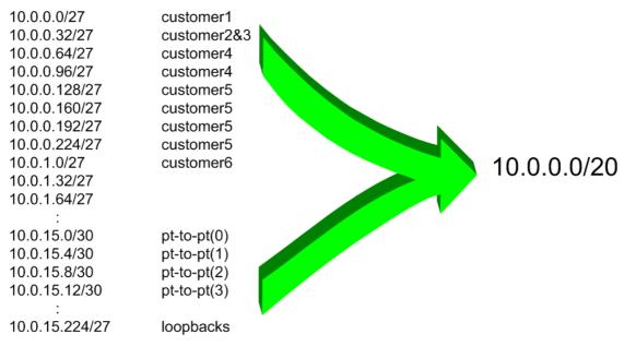
Figure 3 – Extract from an ISP addressing plan
