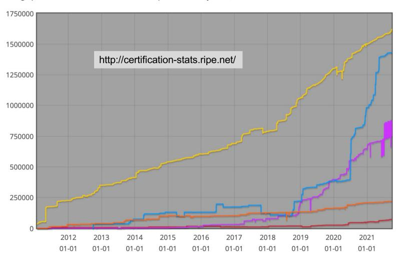
This graph shows the amount of IPv6 address space covered by ROAs, in /32 units
