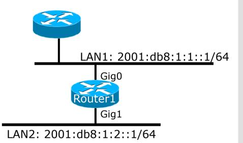
Dual stack IPv4/IPv6 single topology configuration.
