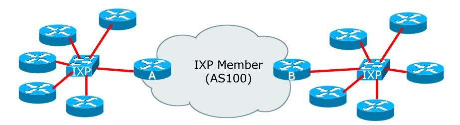
Diagram shows ISP connecting to two different IXPs
