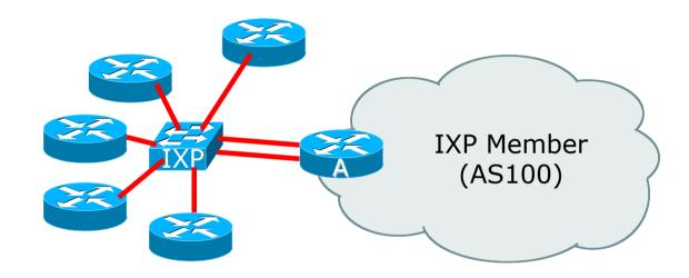
Diagram shows case of two ethernet links from one router
