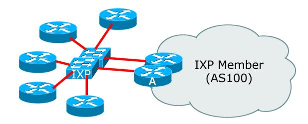
Diagram shows two ethernet links from separate switches to two routers
