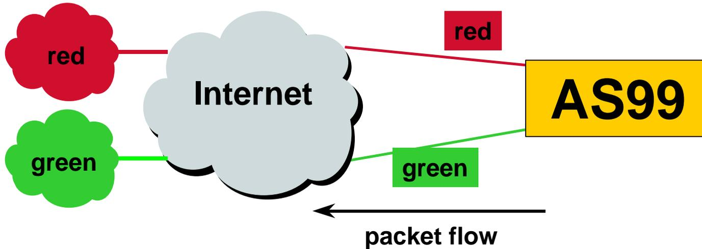
**AS99 uses red link for traffic going to the red AS and green link for traffic going to the green AS**
