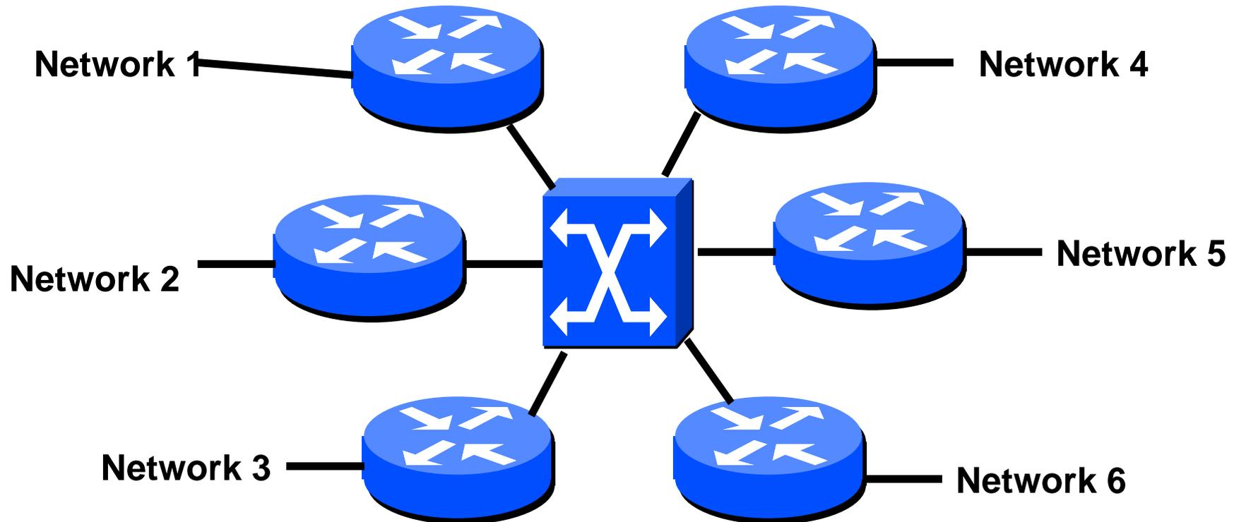
each of these represents a border router in a different autonomous system
