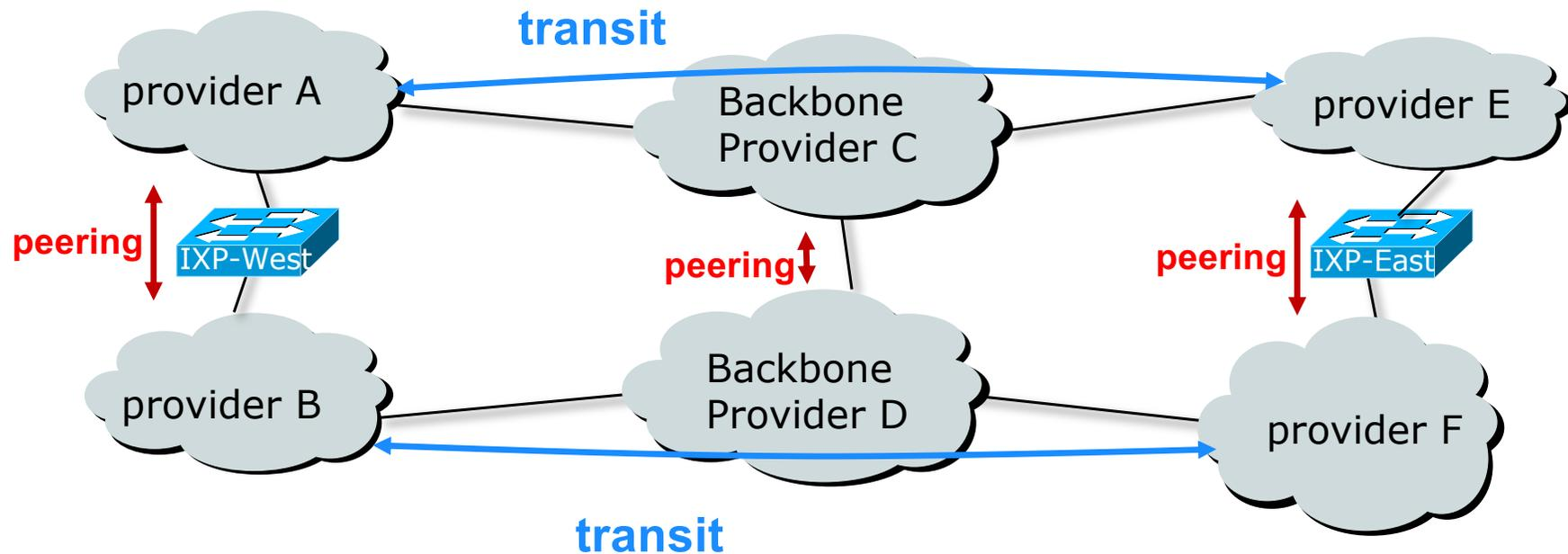
A and B peer for free, but need transit arrangements with C and D to get packets to/from E and F
