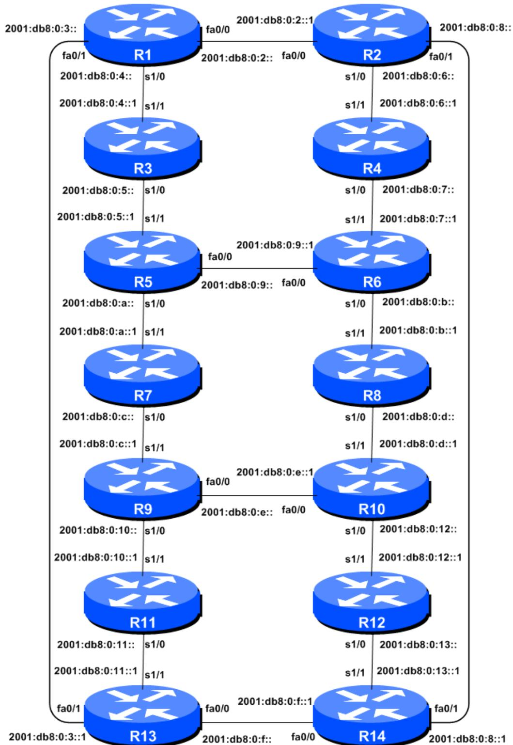
Figure 1 – Addressing scheme for Modules 1 to 5
